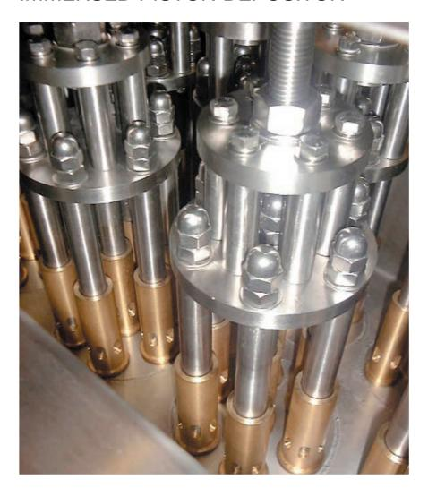
The deposit cylinders are fully immersed in the product to be deposited, within a water or oil heated hopper. Product flows into the cylinder under vacuum, assisted by gravity, and is forced out through a specially designed spring loaded nozzle.
