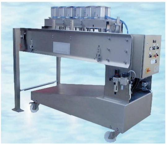
Within the range of depositors offered by the Baynflax Cambridge Range is the immersed piston depositor suitable for use fondant, chocolate or seedless jams.
