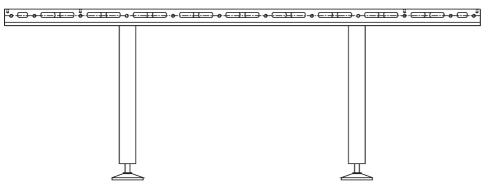
The cooling surface of the Table is fine machined in order to produce a high quality finish. The stainless steel rolled hollow section support legs are height adjustable in order to accommodate any unevenness or slope in the floor level and to provide a perfectly horizontal surface.
