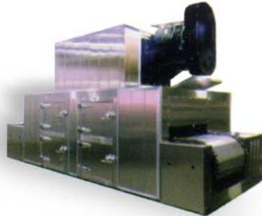
An example of a Babbco Hybrid Oven that was tailored to the needs of a customer is shown in this CAD drawing of a 120-foot oven designed for the production of par-baked frozen products. It combines indirect, direct, and convection oven technology.
